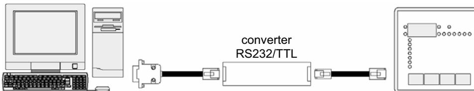
*N.B.:* This type of connection has been designed to be used in the setup, testing or diagnostics phases.
